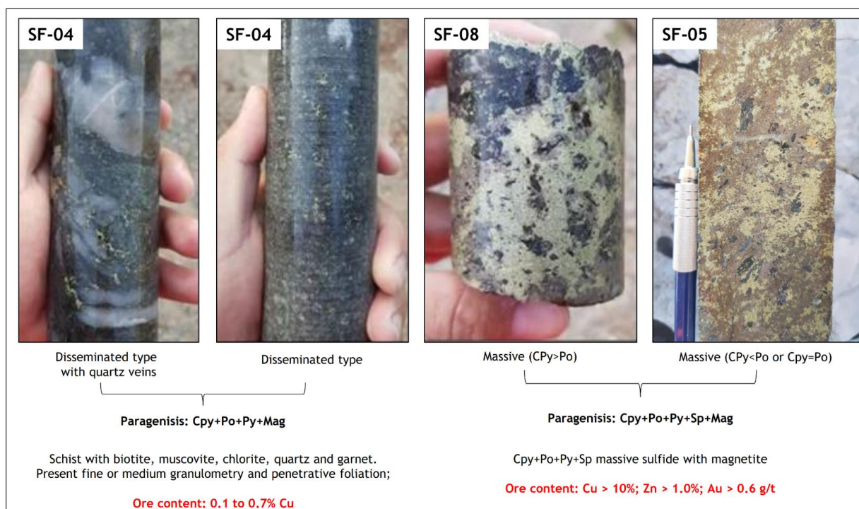
Figure 25.1 Core examples showing disseminated and massive sulphide mineralised zones and interpreted paragenesis. (Prospectiva, 2025).
