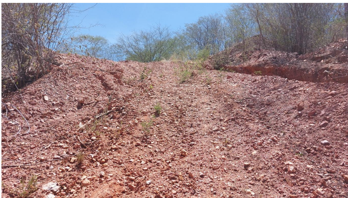
Figure 25.11: Extensive garimpeiro workings on right hand side with mineralised waste rock and colluvium in foreground looking east, which returned samples from metallic screen assays of 3.14 ppm, 5.33 ppm and 13.65 ppm Au for the three colluvial horizons (Selwyn, R. (Jan 2026), conversation with Lewis Harvey)) (source: AMS site visit, 2026).
