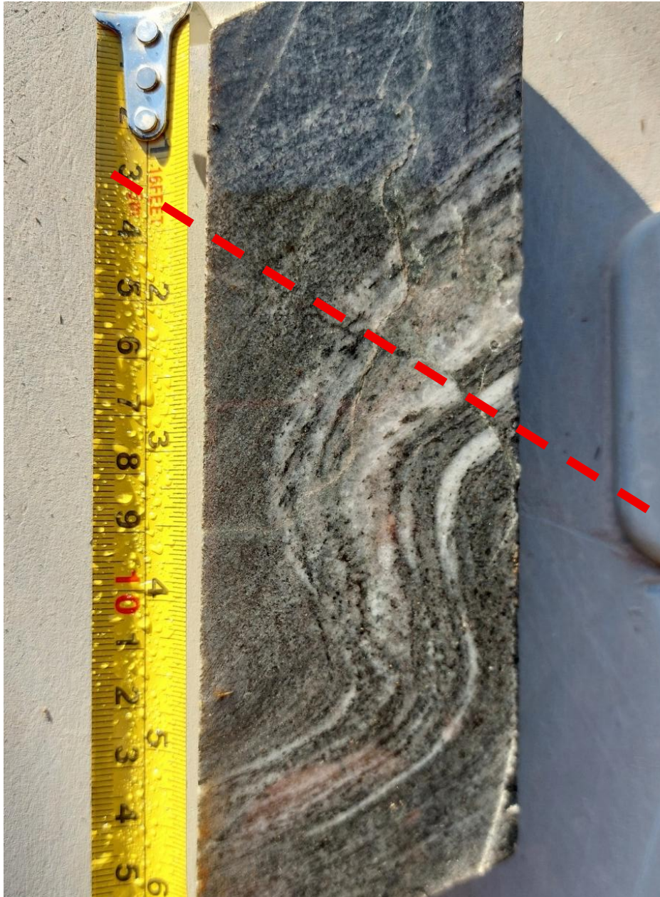
Figure 25.9: TBS_014 at 32.65 to 32.80 metres, showing minor faulting and folding (source: AMS site visit, 2026).
