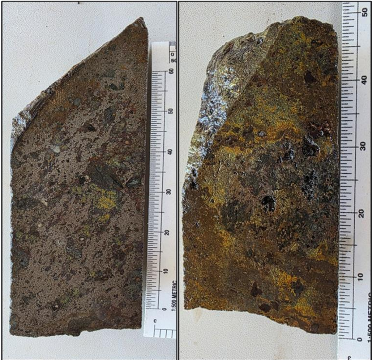
Figure 7.7: Example of massive pyrrhotite-chalcopyrite from drill core. Photo (left) is from SF_005 (a 10-centimetre hand specimen at 45.1-45.2 metres and photo (right) is from SF_006 (a 10-centimetre hand specimen taken at 74.8 to 74.9m) (source: Prospectiva – Drill Core Samples – PMC, 2025).
