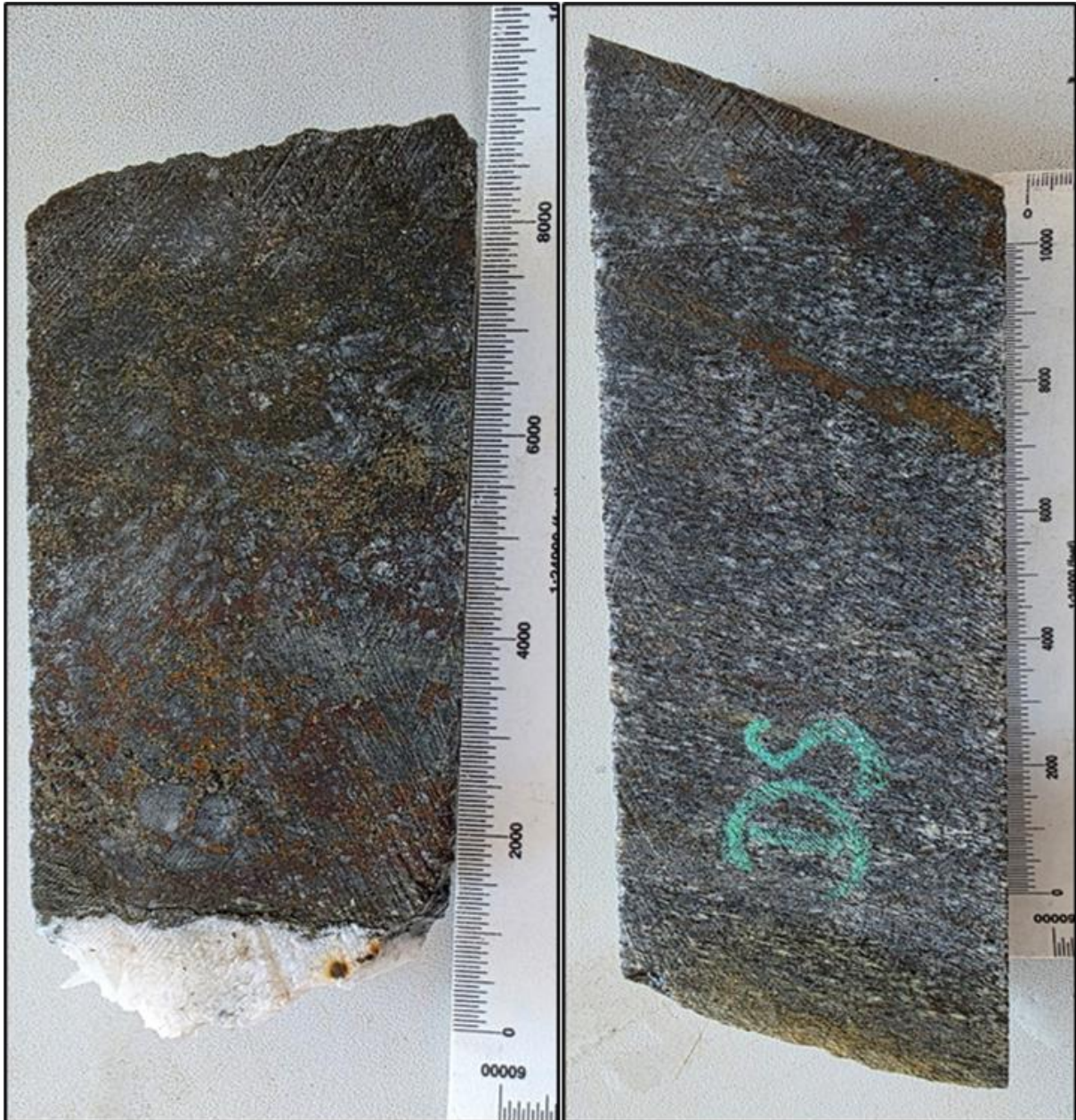
Figure 7.8: Example (left) of semi-massive and distal mineralisation from SF_024 (a 7-centimetre hand specimen taken at 142.15-142.22 and photo (right) of SF_026 (a 15-centimetre hand specimen2 taken at 296.10-296.20m) (source: Prospectiva – Drill Core Samples – PMC, 2025).
