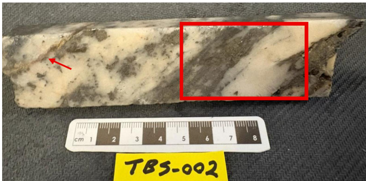
Figure 13.4: Macroscopic view of the core sample and corresponding scanned thin section (TBS-002), with the thin-section location outlined by a rectangle. The core shows strong silicification and well-developed banding, with milky-white quartz-rich ribbons alternating with darker, sulphide-bearing metamorphic laminae. The red arrow indicates a phyllosilicate-rich lamina (source: PMC, 2026).
